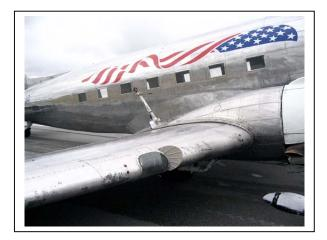
Wherever we put it, it was obviously going to be for a while. My initial inspection told me that at a minimum we had damaged an engine, prop, gear, tire, oil cooler, right wing tip, and complete center section of the whole right wing. How much damage would be found inside the wing was anyone's guess.
