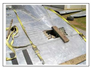
Next came the process of cutting away all the scrap and bent aluminum. It looked like an explosion had occurred in the center section of that wing. These were long days spent trying to figure out if this was a fixable airplane or not.
