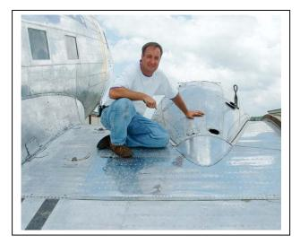
So we shot about 500 or so of these rivets into this particular corrugation repair and finally, the corrugated part was all done.
